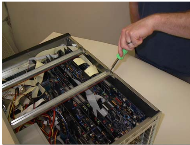
Figure 1.8: Removing the Retaining Bars
