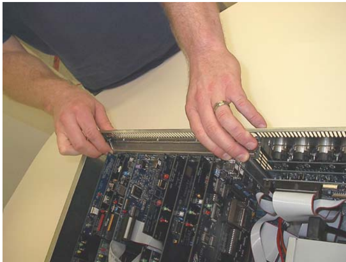
Figure 1.11: Pushing Down on the Rear Lock-down Panel
